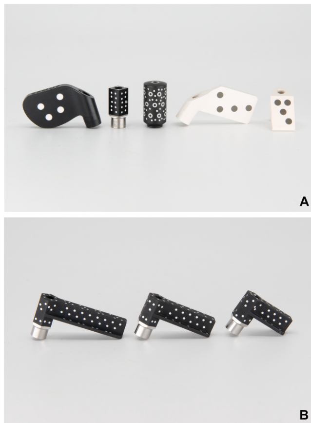
Figure 7. A, Markers of extraoral photogrammetry systems tested. B, Implant scan bodies of intraoral photogrammetry system.
